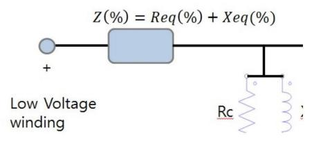
• Equivalent Series Impedance Z(%) of Double Winding Transformer :
