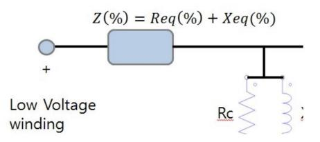
• Equivalent series impedance between low voltage windings :
